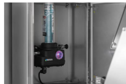
Automatic Lubrication Centralized lubrication system with automatic grease distribution.
