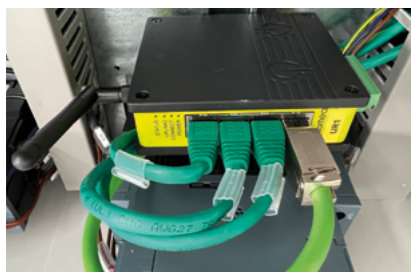
Online remote Access Integrated modem to enable remote access for Pujolàs technical service. Usable through either cable or Wi-Fi connection.
