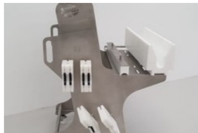
Cleaning Trolley The cart is made of stainless steel for easy disassembly of molds and proper storage.
