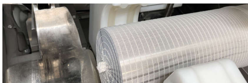
Net dispenser An innovative system that fully compacts the meat in the extremities, resulting in a higher yield product.
